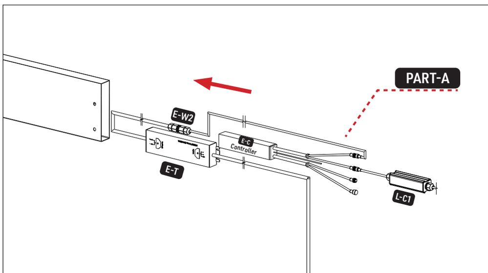
The wire of transformer go through post and wire come out from drain, "INPUT" connect home power, "OUTPUT" connect LED .
