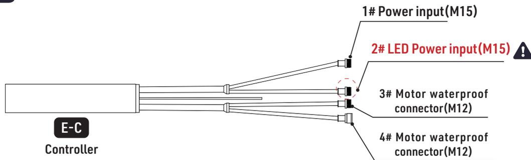
Connect LED controller to Transformer (PART-A) firstly, then place it in cavity of beam.
